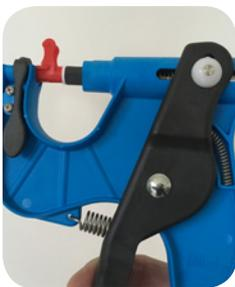
2c. Carefully squeeze the plier handles until the large piston comes to a stop against the red connection piece
