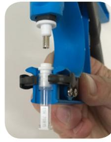
**2a.** Remove the TSU tube from the pliers by squeezing the two spring loaded clips together, then slide out the tube.
