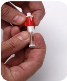
1. Take an assembled TSU (needle + connection piece + collection tube)
